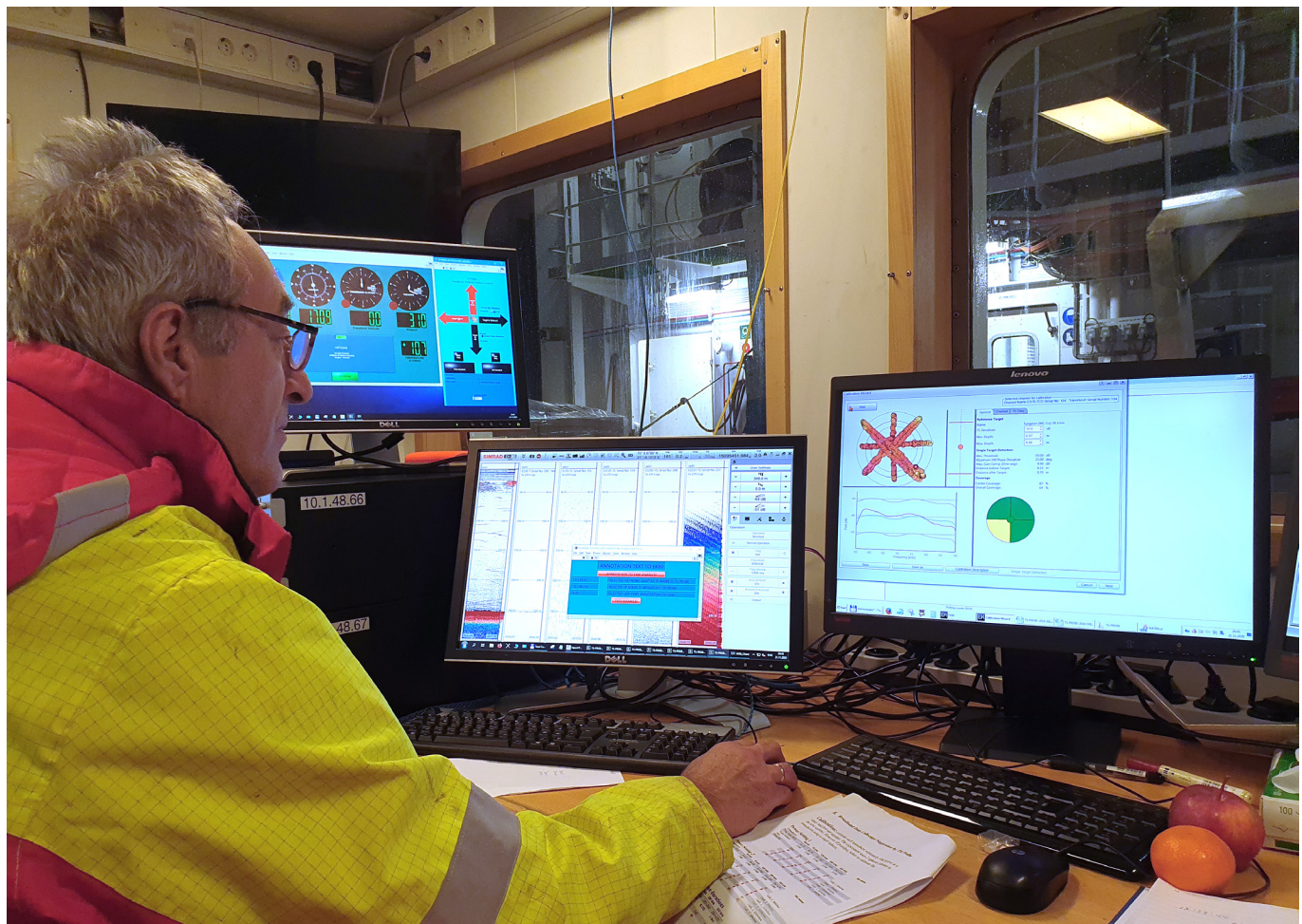
Figure 4. Operation during calibration of the target strength probe used to obtain broad banded spectrum of individual targets..
