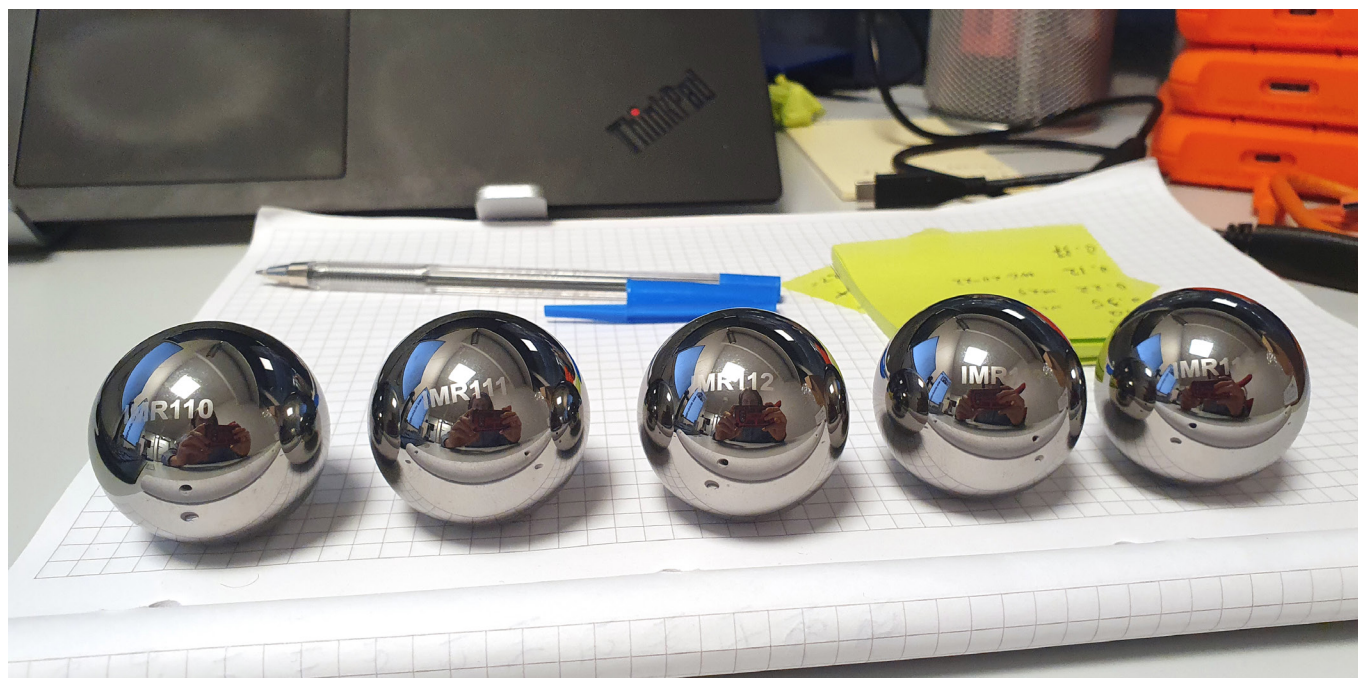
Figure 1. Spheres for broad band calibration.
